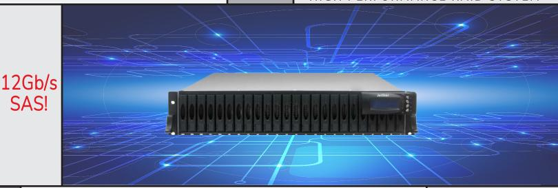
The JetStor SAS Model 824S Direct Attached Storage (DAS) array features 12Gb SAS host performance to increase system efficiency and performance. This DAS storage system supports optional dual controllers and is equipped with 24 hot swappable SAS2/SATA3 hard disk drive bays with fast SAS2 host channels for a rapid, uninterrupted access to your most demanding applications requiring either high bandwidth or very rapid random I/O performance.
