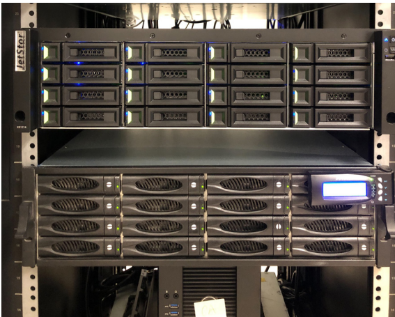
JetStor 816iXD iSCSI SAN storage system (top) and JetStor 716iSD storage array (bottom)
